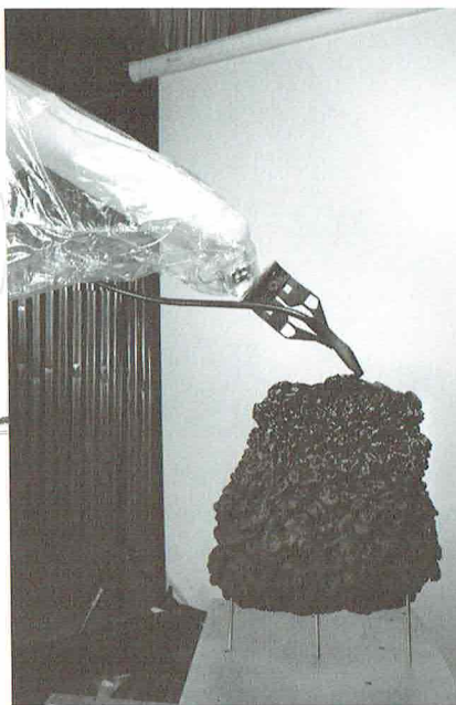
MMYST. LABORATORY TEST OF ROBOTIC EXTRUDER ARM USING STARCH-BASED BIOPLASTIC.
